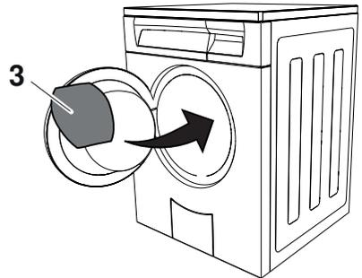
**Inserting the door filter / door filter mat**
