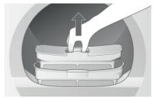
▶ Pull out the inner, fine filter **A** and swing it open.
