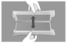
▶ Pull out the outer coarse filter **B** and swing it open.
