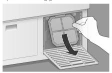
Remove the air filter D by pushing it slightly upwards and then pulling it diagonally downwards.
