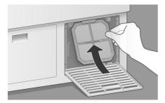
► Replace the air filter and close the cooling grid.
