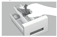
Release the blue insert in compartment by lightly lifting it up and take it out of the detergent drawer.
